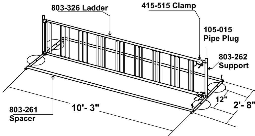
Main Frame, legs and spacers are 1 5/8" O.D. hot galvanized welded pipe with 3/4" O.D. hot galvanized ladder rungs. Spacing between tire posts is 3" center-to-center for small gap, 8 1/2" center-to-center for large gap.
